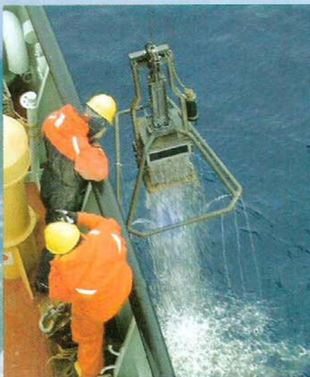
A large sediment corer being recovered after collecting the sample of deep ocean floor (left)
