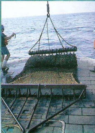
A Scallop Dredge on the NOAA research ship, Oregon II, used to sample marine life along sea floor (left)
